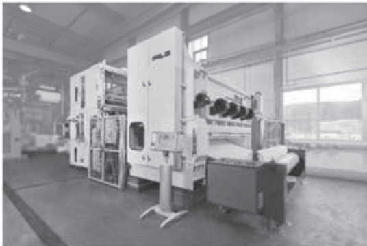
“Hypertex” Technology, combination of Scrim fabric machine (background, OnTec) and needle loom (foreground, DILO)
